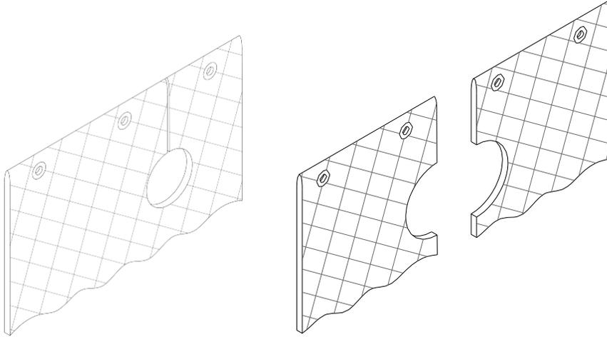
Please note that the relief cut from the curtain edge to the penetration can affect the support of the curtain below the cut.
