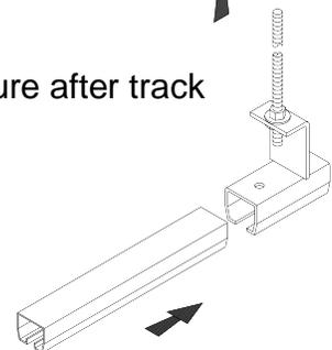
The track assembly should be level  $\pm \frac{1}{4}$  " .
