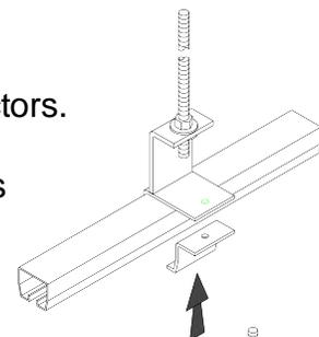
**For slide through brackets with set screw**
